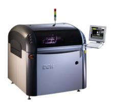
The change of squeegee pressure has a significant impact on printing. Too small pressure will make the solder paste unable to effectively reach the bottom of the stencil opening and not be well deposited on the pad. Too much pressure will cause tin The paste is printed too thin and can even damage the stencil.
